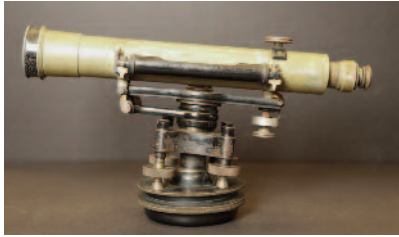
SURVEYING LEVEL USED BY FERNANDO TORRAS, ENGINEER OF THE BRUNSWICK-ST. SIMONS CAUSEWAY C. 1920. MANUFACTURED BY BAUSCH AND LOMB OPTICAL CO. GIFT OF ROBERT TORRAS, SR., SON OF FERNANDO.
